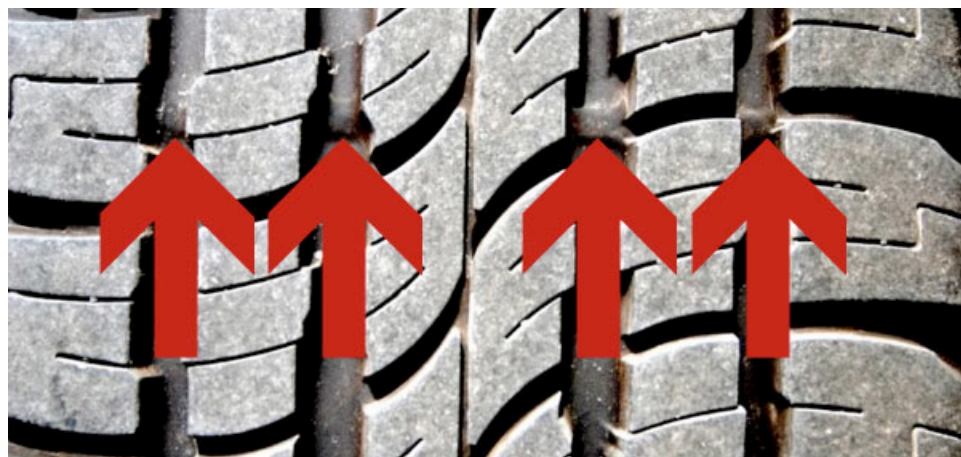
Enlarged image of a tire tread shows characteristics unique to the mold used to create this tire (red arrows). (Courtesy of John Black, Ron Smith & Associates)
